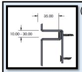
(Artisan Plank) (ART-PLA 35mm )(Structural plank) for materials 1mm to 3mm +
