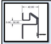
(Artisan Plank) (ART-PLA 42mm) (Maxi plank) for materials 1mm to 3mm thick
