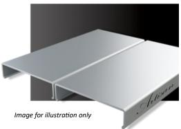
**Panel dimensions (std);** - **Width** = 100mm up to 650 mm (For flat unstiffened panel depending on substrate, gauge and required aesthetic.) 100 - 300 = 1mm / 100 - 550 = 2mm / 100 - 650 = 3mm. (Based on MCRMA recommendations for Aluminium)
